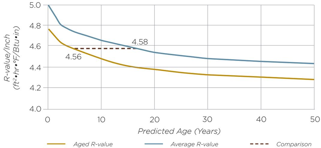
Applying ASTM C1303, a sample of XPS insulation obtained commercially was evaluated and the predicted aged R-value determined. A comparison was made between the 5-year (point-in-time) aged R-value and the 15-year average R-value to demonstrate their equivalence as noted in ASTM C1303, Section 5.4. The 5-year aged R-value of 4.56 agreed quite well with the 15-year average R-value of 4.58 (see chart above).
